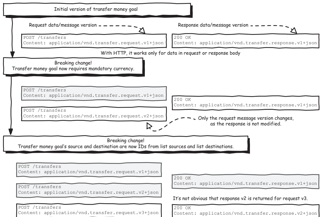
Figure 9.14 Data (or message) versioning with content negotiation
